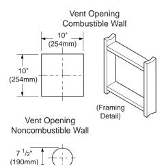
Figure 12 - Vent Opening Requirements
